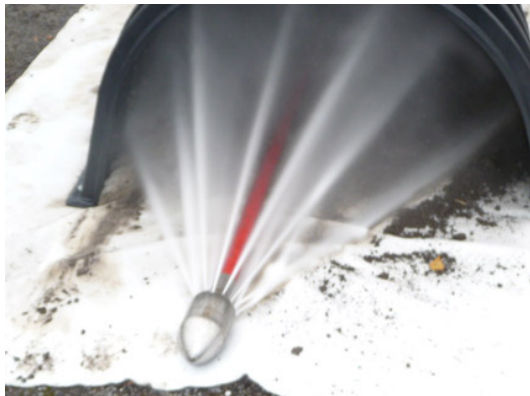
Image 3: Flushing nozzle with reverse conical jets
